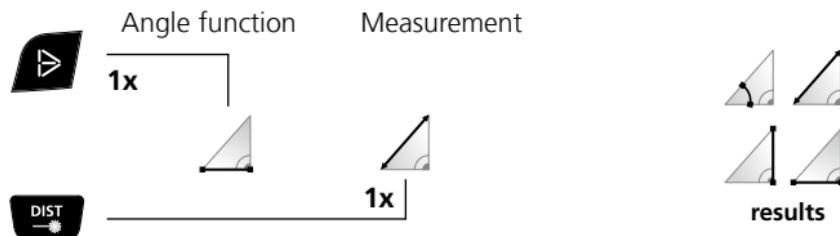
The measurement results are determined automatically by the 360° inclination sensor.
