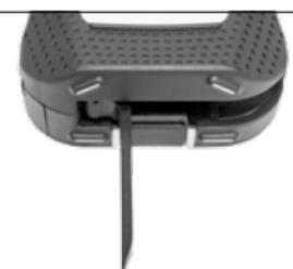
For stop measurements move the pin to the side and select the „measurement plane REAR“ setting.
